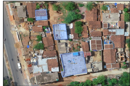
2D measurement for planning on a drone orthomosaic
